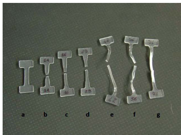
Figure 13. Evolution of type of fracture with temperature: untested sample (a), -40^\circ\text{C} (b), -20^\circ\text{C} (c), 0^\circ\text{C} (d), 23^\circ\text{C} (e), 40^\circ\text{C} (f), and 60^\circ\text{C} (g). [Color figure can be viewed in the online issue, which is available at wileyonlinelibrary.com .]
